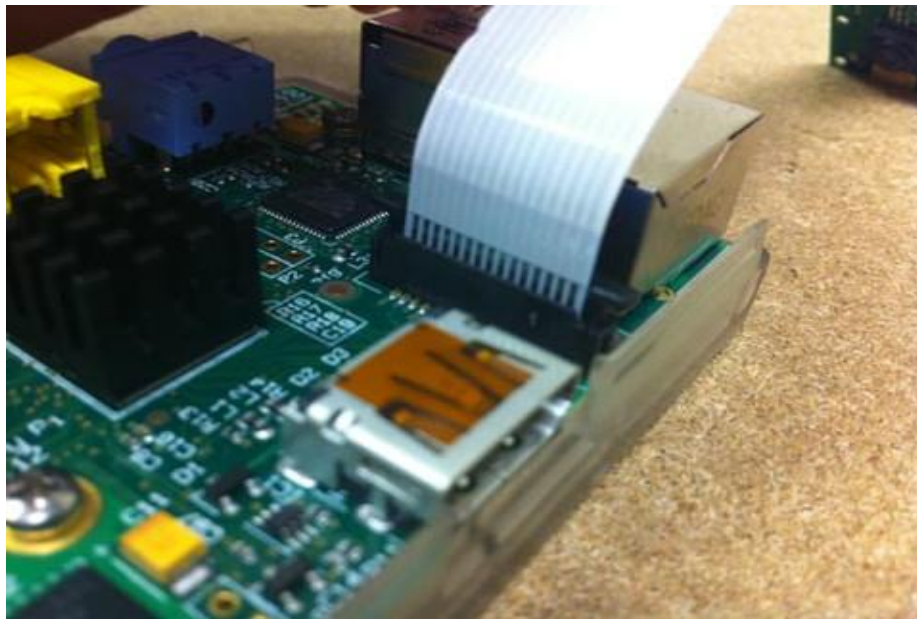
Figure 3.12: Raspberry Pi camera module connected to CSI port
